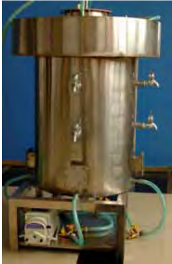
Figure 5. Photo of Two-phase Digester
