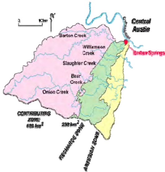
Figure 2. Barton Springs Aquifer showing (right to left) the confined (artesian), recharge, and contributing zone (from Budge and Sharp, 2008).
