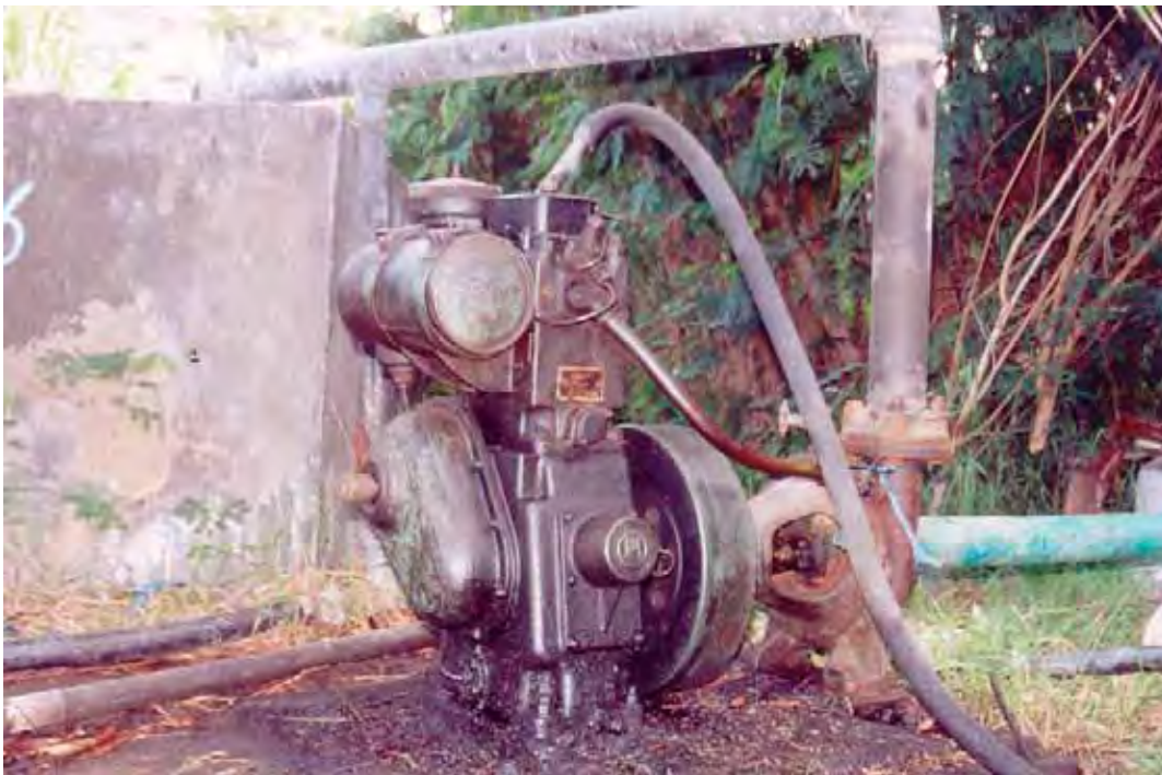
Figure 5: Photo showing a diesel machine pump used in old farms in the eastern part of the UAE. Note that these diesels are associated with dug wells (Photograph by Ahmed A. Murad, March of 2002).
